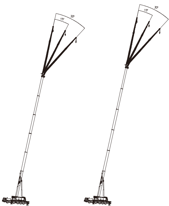
Main boom: 59.6m, Jibs: 24.5m (17.5m + 7m jib extension) Main boom: 64.0m, Jibs: 24.5m (17.5m + 7m jib extension)
