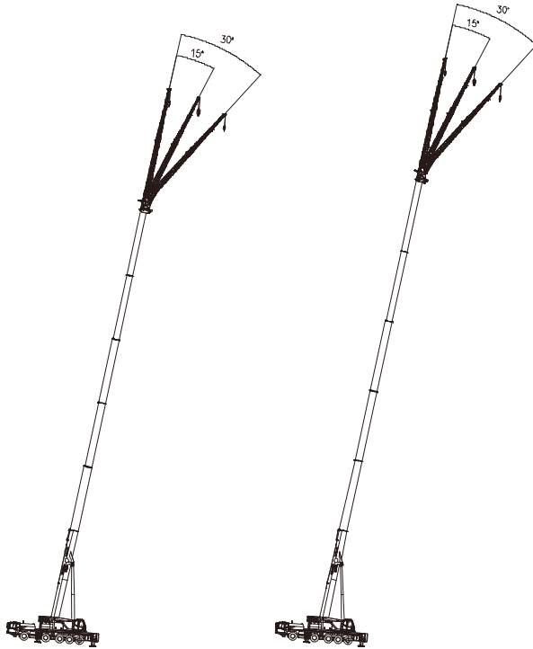
Main boom: 59.6m, Jibs: 17.5m (10.4m + 7.1m jib section 2) Main boom: 64.0m, Jibs: 17.5m (10.4m + 7.1m jib section 2)
